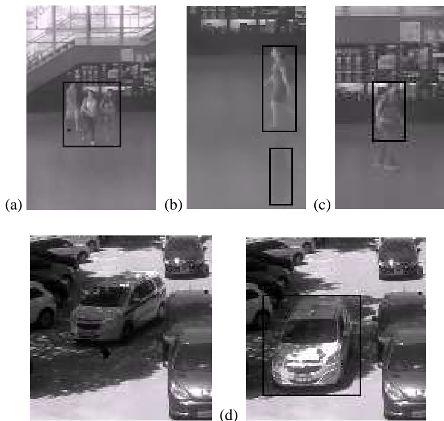
Figure 8 - Detection errors that can generate false alarms: (a) Object occlusion, (b) reflex, (c) low contrast and (d) shape changes.
