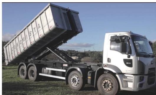
Figura 2.9: Roll-on roll-off
